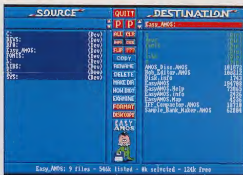
Easy AMOS has a directory utility which allows you to access files without using the CLI.
